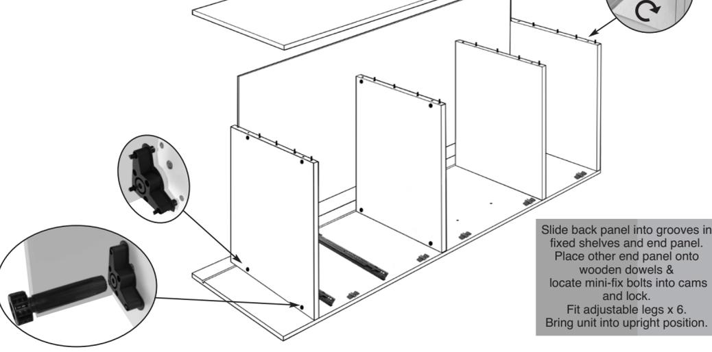
**6** Bring unit into position were it is to be fitted and level in all plains, place 'L' shape brackets provided onto top shelf and secure. Secure unit to wall, screws cannot be provided because of difereing wall materials. When unit is securely fitted in position firmly push shelf supports into pre-bored holes in end panels. **IMPORTANT.** When adjusting the height of the unit make sure that the legs are not adjusted below the nominal 140mm plinth height.
