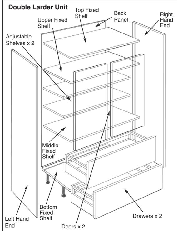
Note: It is strongly recommended that the unit is secured to the wall prior to Doors, drawers & adjustable shelves being fitted.
