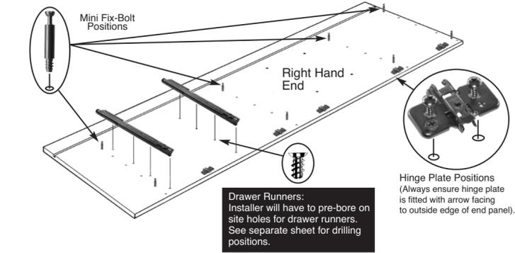
**3** Locate Top, Middle & Bottom Shelf, onto Wooden Dowels & Mini-fix Bolts & Lock
