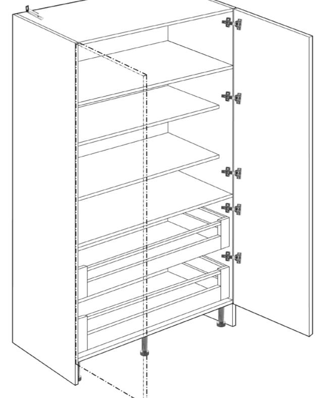
Place shelves onto shelf supports and firmly press home. Bring drawers into position on runners and push home. Bring doors into position locate clip-on hinges onto hinge plates. (See clip-on hinge adjustment opposite for alignment details).
