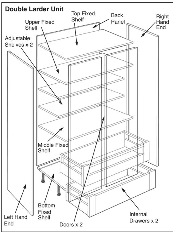
Note: It is strongly recommended that the unit is secured to the wall prior to Doors, drawers & adjustable shelves being fitted.
