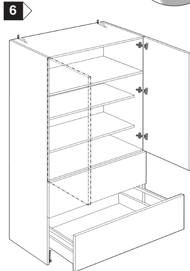
Place shelves onto shelf supports and firmly press home. Bring drawers into position on runners and push home. Bring doors into position locate clip-on hinges onto hinge plates. (See clip-on hinge adjustment opposite for alignment details).
