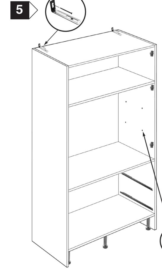
Bring unit into position where it is to be fitted and level in all plains, place 'L' shape brackets provided onto top shelf and secure. Secure unit to wall, screws cannot be provided because of differing wall materials. When unit is securely fitted in position firmly push shelf supports into pre-bored holes in end panels.
