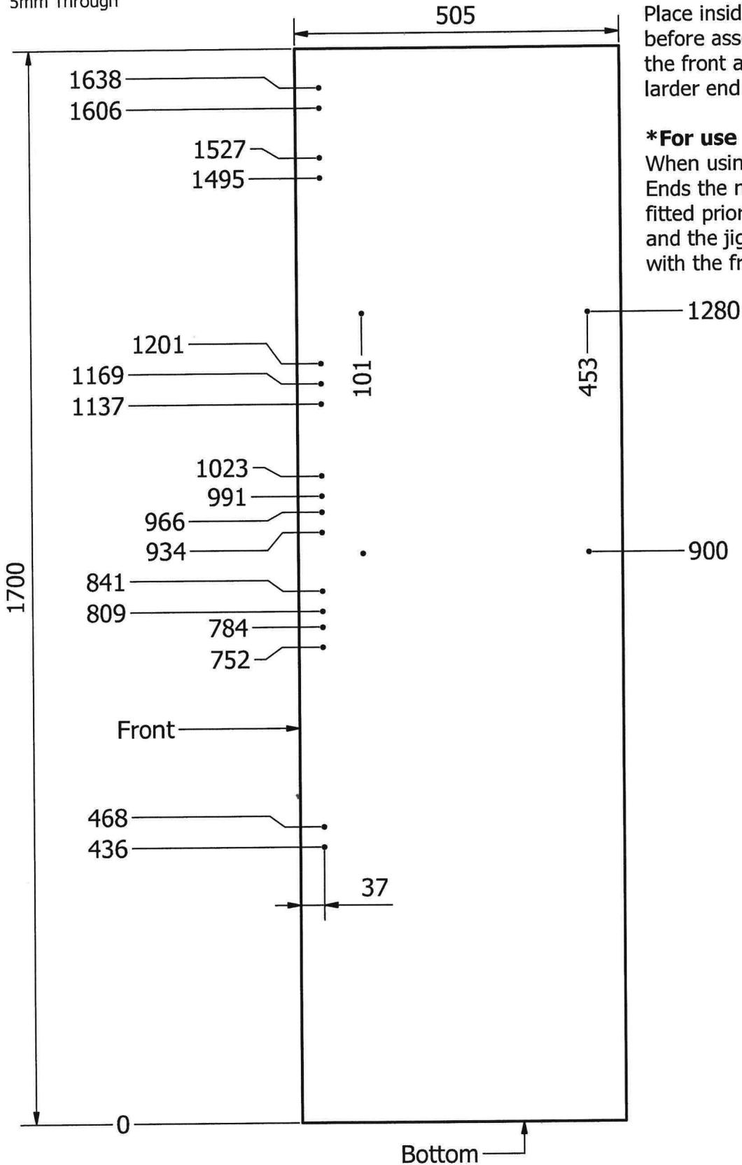
Place inside larder unit end before assembly, level with the front and bottom of the larder end
