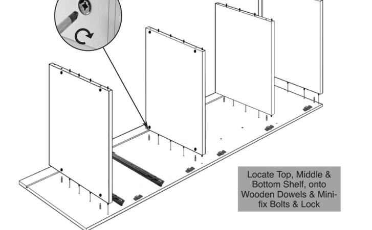
**2** Mini-fix cams are fitted to underneath. Groove for back panel is inside cabinet
