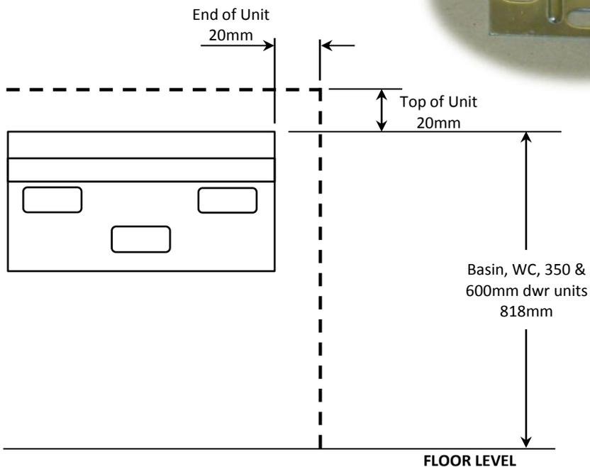
**Installation Note** - All edges should be fully sealed taking special care with work surface joints and edges, around basins and especially bath panels.
