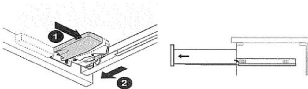
Insertion - Keep drawer base square to runner & push back, it will automatically lock in place.
