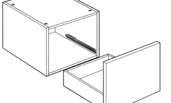
Once drawer front is fitted to drawer box bring drawer into position and place onto fully extended runners. Ensure drawer runner locates into the rear of the drawer box (small pre drilled hole). Firmly close the drawer into the unit. The drawer should locate If required unused pre bored holes in end panels can be plugged using 5mm cover caps
