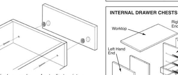
Firmly press drawer front adjusters into prebored holes in drawer front, bring drawer box into position and secure to drawer front with screws provided through pre-bored holes in drawer box.
