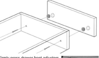
Firmly press drawer front adjusters into pre-bored holes in drawer front, bring drawer box into position and secure to drawer front with screws provided through pre-bored holes in drawer box. Turn drawer over and fit drawer runner brackets to underside of drawer box with screws provided as shown below.
