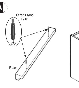
surface with pre-bored holes facing upwards. Fix Large Fixing Bolts into positions indicated.
