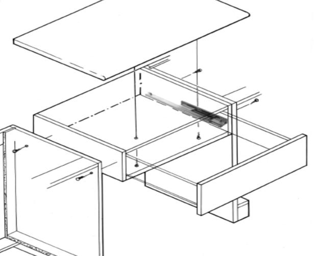
The dressing table should be positioned between two units and secured with either connecting bolts (these are supplied) or screws. It is left to the installer to decide on the position of the holes which require drilling to secure the units Worktop can be secured to unit using 2 x 30mm screws provided. Prior to fitting it will be required for installer to drill holes in top shelf where required. Bring screws into position and secure
