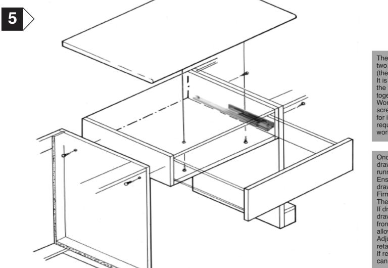
The dressing table should be positioned between wo units and secured with either connecting bolts (these are supplied) or screws. t is left to the installer to decide on the position of the holes which require drilling to secure the units crews provided. Prior to fitting it will be required for installer to drill holes in top shelf where required. Bring screws into position and secure
