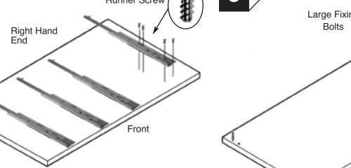
Lay end panels for drawer runners face down on rotective surface. Bring Drawer runners into position and fix to end panels to pre-bored holes with runner screws. Repeat operation for Left hand end panel.
