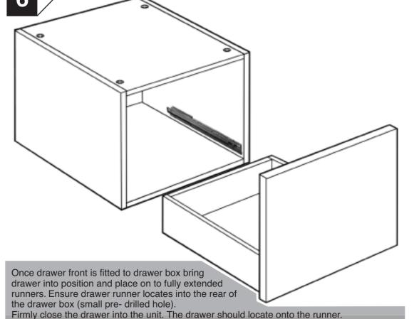
drawer fascia adjustment is required, slacken drawer fascia retaining screws. Within the
