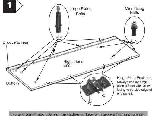
Lay end panel face down on protective surface with groove facing upwards. Fix Large Fixing Bolts, Mini Fix Bolts & Hinge Plates into positions indicated. Repeat operation for Left Hand End Panel.
