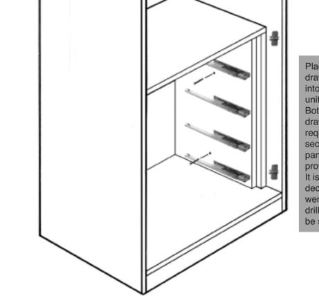
Place end panels with drawer runners fitted into position against unit end panels. Both end panels with drawer runners fitted require to be secured to unit end panels with screws provided. It is left for installer to decide on position were holes are to be drilled for screws to be secured.
