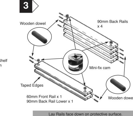
ensuring arrow on cam faces outwards. mly press home wooden dowels into pre-bored holes NB: All back rails and back rail lower are 90mm deep, the front rail is 60mm deep. Always ensure the ont rail is placed in the correct position when assembling
