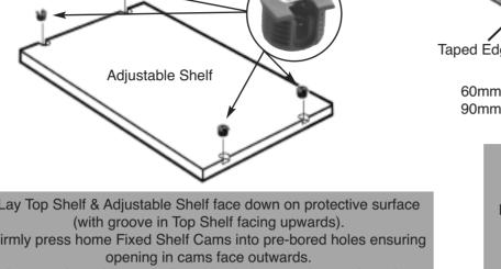
Firmly press home Mini Fix Cams into pre-bored holes ensuring arrow on cam faces outwards. rmly press home wooden dowels into pre-bored holes, ensuring they are fully knocked in. NB: All back rails and back rail lower are 90mm deep, the front rail is 60mm deep. Always ensure the front rail is placed in the correct position when assembling
