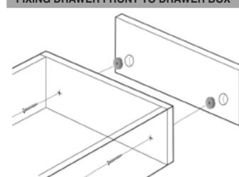
Firmly press drawer front adjusters into prebored holes in drawer front, bring drawer box into position and secure to drawer front with screws provided through pre-bored holes in
