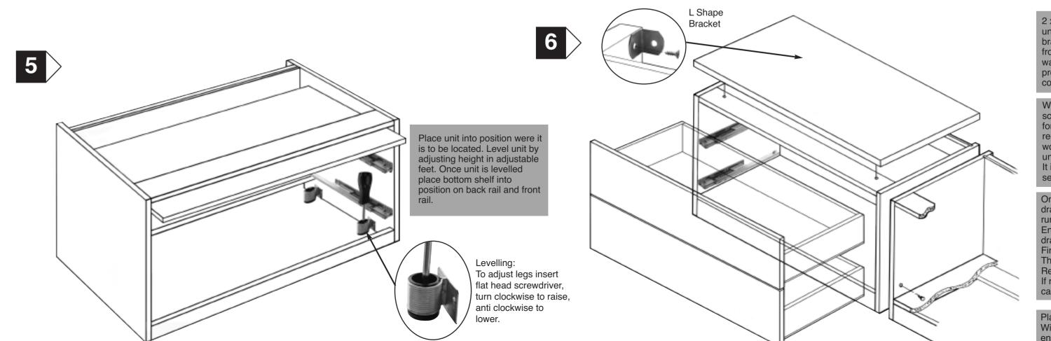
2 x 'L' shaped brackets are supplied for securing unit to wall or securing worktop to unit. If using rackets to secure worktop these will be placed in ont of back panel. If using brackets to secure to wall position as indicated. Screws cannot be provided for securing to wall due to differing wall
