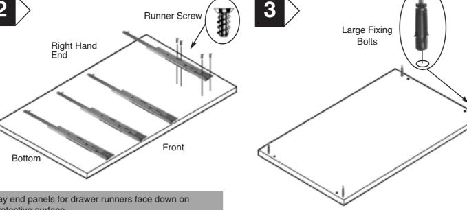
ay end panels for drawer runners face down on otective surface. ring Drawer runners into position and fix to end panels to pre-bored holes with runner screws. epeat operation for Left hand end panel.
