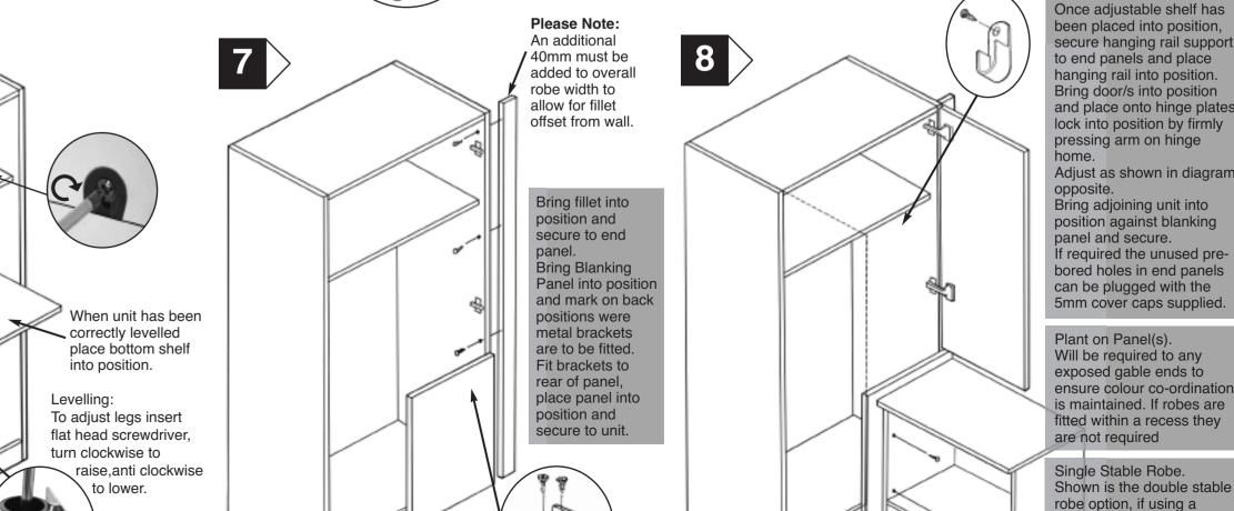
ecure hanging rail suppor to end panels and place anging rail into position. ring door/s into position nd place onto hinge plate: ock into position by firmly pressing arm on hinge Adjust as shown in diagram Bring adjoining unit into position against blanking panel and secure. If required the unused prebored holes in end panels
