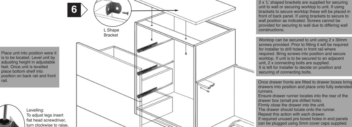
drawer box (small pre drilled hole). Firmly close the drawer into the unit. The drawer should locate onto the runner. Repeat this action with each drawer. required unused pre bored holes in end panels can be plugged using 5mm cover caps supplied.
