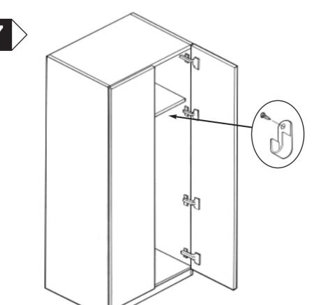
position, secure hanging rail support to end pane and place hanging rail Bring door/s into position and place onto hinge plates, lock into position by firmly pressing arm o ninge home. Adjust as shown in agram opposite. required the unused e-bored holes in end panels can be plugged with the 5mm cover caps
