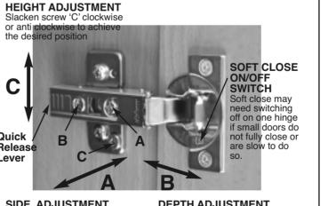
SIDE ADJUSTMENT Adjust screw 'A' clockwise or desired position.
