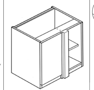
Prior to fitting corner post please ensure that the correct handing of door has been decided. Failure to do so could result in unnecessary damage
