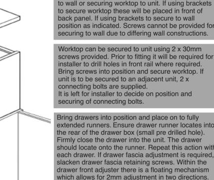
Adjust as necessary and tighten drawer fascia f required unused pre bored holes in end panels car be plugged using 5mm cover caps supplied.
