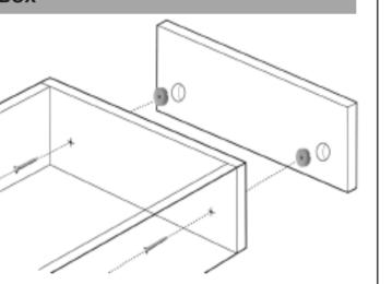
Firmly press drawer front adjusters into prebored holes in drawer front, bring drawer box into position and secure to drawer front with screws provided through pre-bored holes in drawer box.
