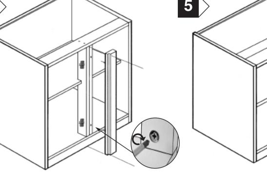
Bring corner post into position and secure to inner corner post as own. Ensuring all Mini-fix cams are locked fully. s the internal space is reduced by the internal corner post the ustable shelf will require scribing around the internal corner post, nce this has been completed bring adjustable shelf into position and y press down onto Mini-fixing bolts. Fully lock all Fixed shelf cams.
