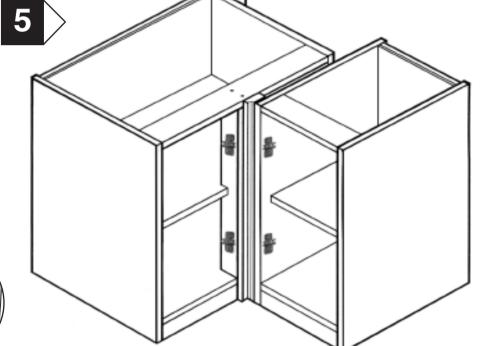
Place unit into position were it is to be located. Ensuring gap to wall is correct to size of door being used, (see diagrams below for spacing details). ring adjoining unit into position as shown and secure to corner post with
