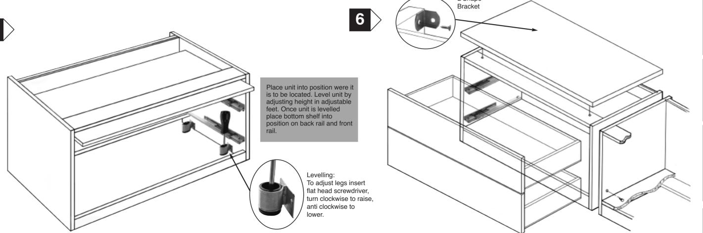
2 x 'L' shaped brackets are supplied for securing init to wall or securing worktop to unit. If using rackets to secure worktop these will be placed ir front of back panel. If using brackets to secure to wall position as indicated. Screws cannot be provided for securing to wall due to differing wall
